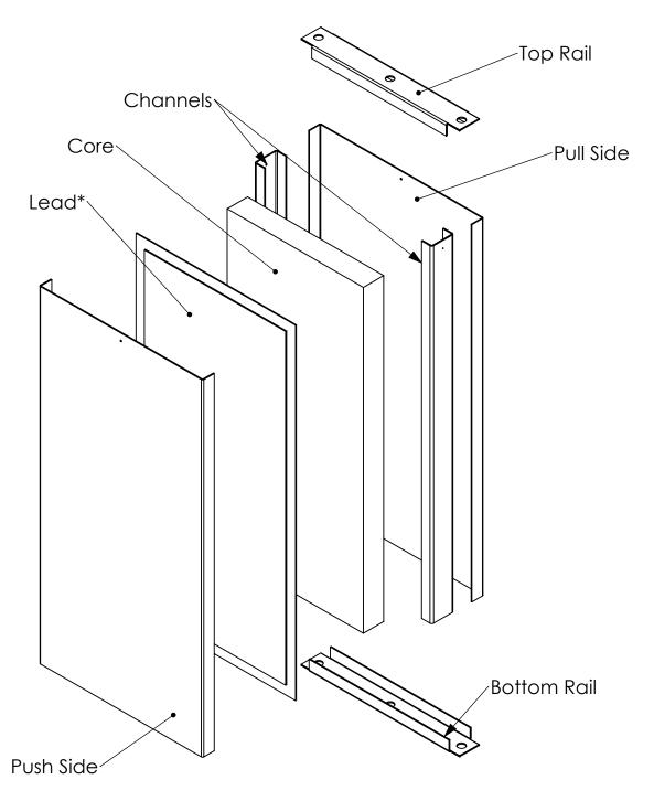
\*Lead glued to push side unless otherwise specified \*Lead glued to core
