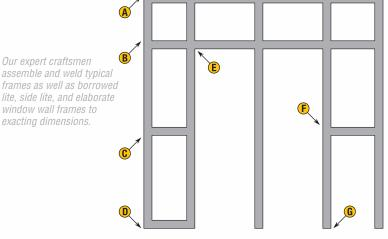
**Corners** – Corners can be supplied face-welded and ground smooth, or full-throat back welded. Pharmaceutical grade throat welded for DefendDoor stainless steel.
